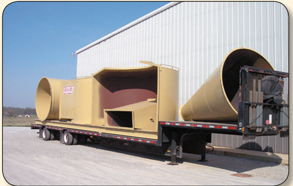
15' dia. Cyclone sectioned with flanges for shipping purposes.
