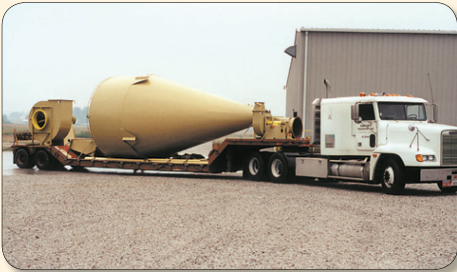
All welded oversized cyclone being delivered with main fan and relay fan.
